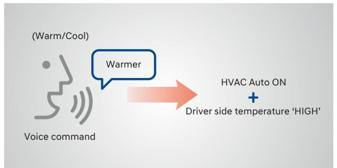
Vehicle functions can be controlled with voice commands. Integrated vehicle control and activation is possible with a single voice command.
