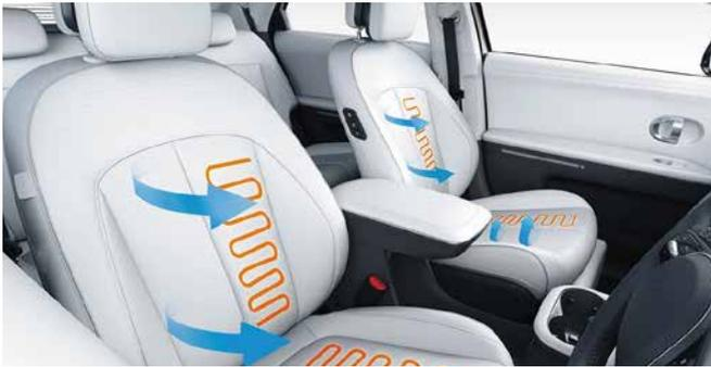
Premium relaxation seats may include heating and cooling features. These features allow the occupant to alter the seat temperature to their liking, improving overall comfort regardless of the weather.
