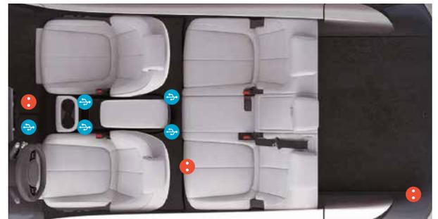
Front : 2 USB chargers, 1 USB port for data support, 1 power outlet.
