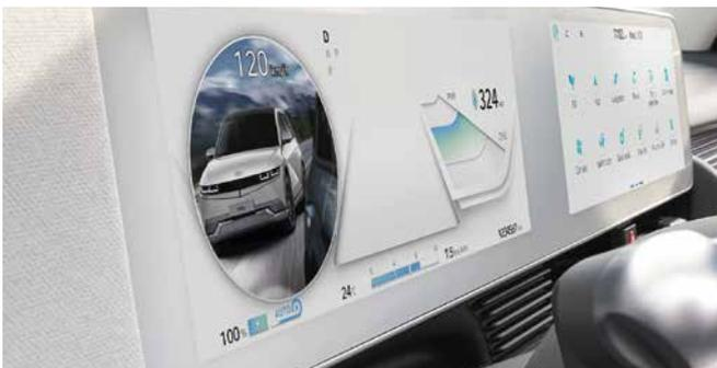
Blind-Spot View Monitor displays video of the blind-spot view for a safe lane change. When operating the turn signal switch, BVM displays video of the blind-spot view for the direction indicated.
