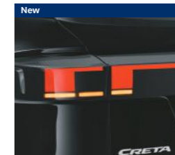
LED rear turn signal with sequential function
