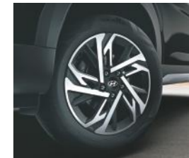
R17 (D=436.6 mm) Diamond cut alloys
