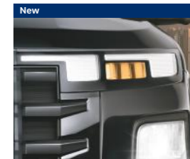
Front turn signal with sequential function
