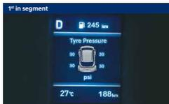
Tyre pressure monitoring system (TPMS) - highline
