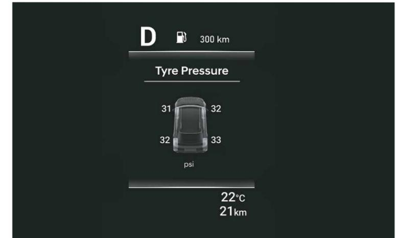
Tyre pressure monitoring system (Highline)
