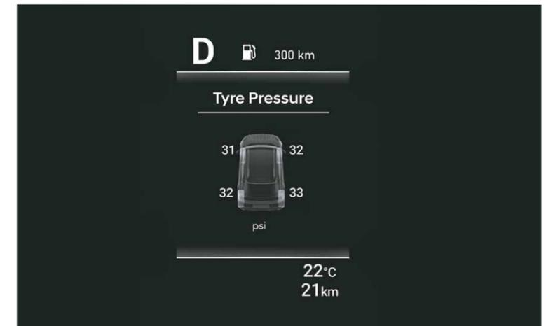
Tyre pressure monitoring system (Highline)
